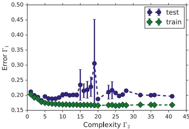
FIG. 14. Solar power study, average Pareto front obtained using GP: with increasing complexity, training and testing data first behave similarly, then testing deviates strongly indicating overfitting or too small testing data set, respectively. The peaks around complexity 20 are due to two reasons: there are only a few models on the fronts (1–3), and one of them is an extreme outlier.
