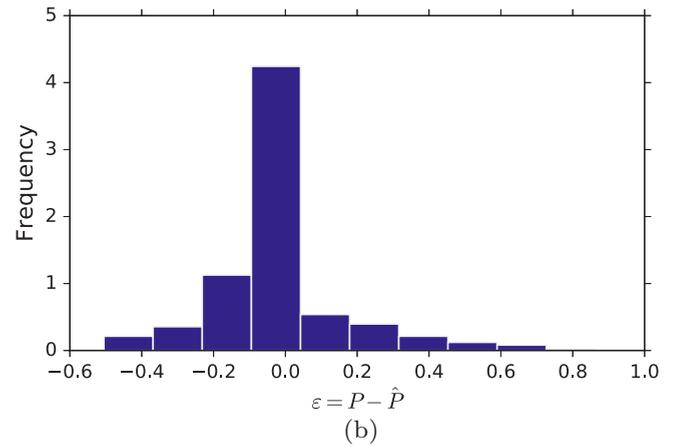
FIG. 15. Solar power study, method GP. (a) Real and predicted time series. We display the results of the first week of August 2015. Prediction used model of complexity 4 which had lowest error on the test set. (b) Histogram of the residuals  $\varepsilon = P - \hat{P}$ . The distribution is asymmetric around zero. The model tends to underpredict.
