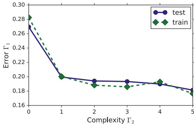
FIG. 12. Solar power study, Pareto front obtained using FFX. The results for FFX are as accurate as the ones obtained with GP. Test and training set are, however, nicely aligned. This demonstrates not only consistency of the models, but less variability of the models found.
